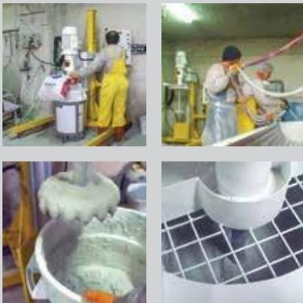
ASE MIX 3 and ASE MIX 5 are modern mixers designed to achieve the most suitable mortar admixture required for GRC applications.
